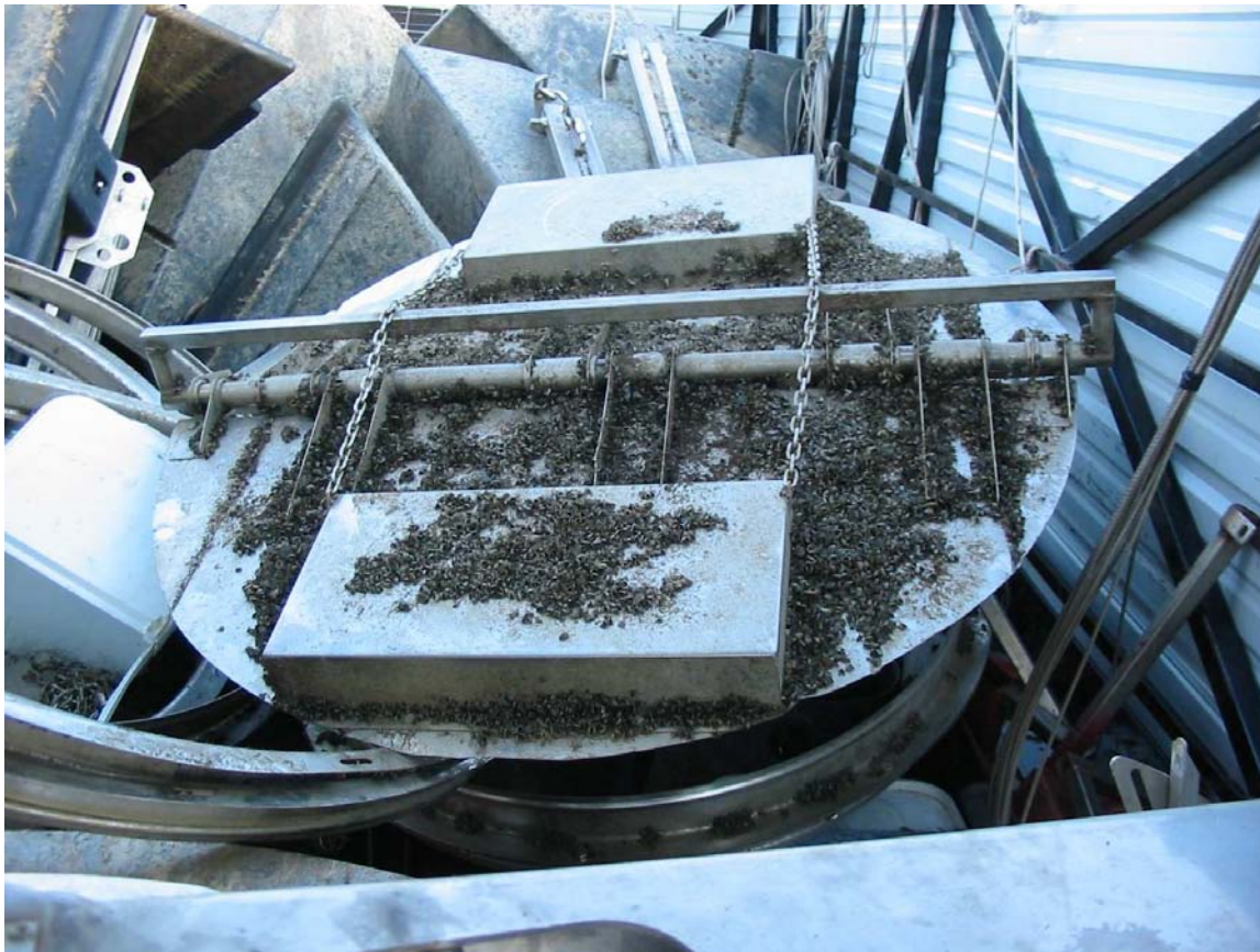
Figure 1. Thousands of zebra mussels were found on a pump unit that was en route to North Dakota from Vermont.
